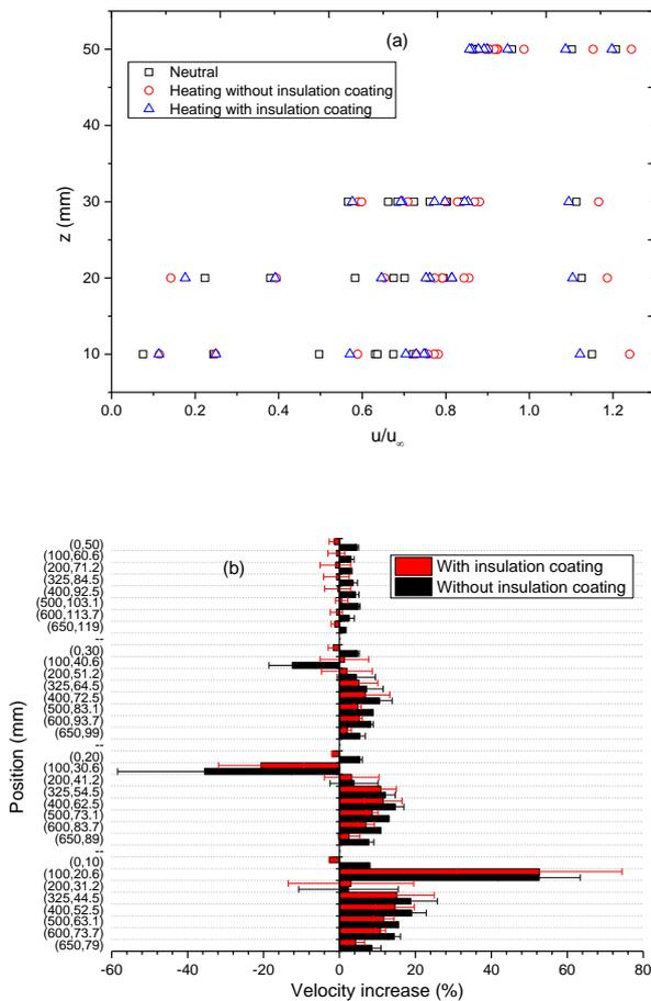
Fig. 7 Velocity (a) and velocity increase (b) at each layer after heating the rooftop, with and without insulation coating
