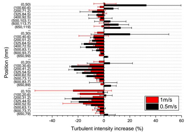
Fig. 5 Turbulent intensity increase at each layer after heating the rooftop
