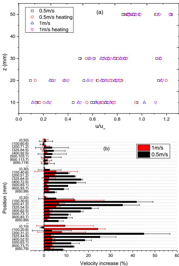
Fig. 4 Velocity (a) and velocity increase (b) at each layer after heating the rooftop
