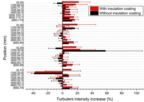
Fig. 8 Turbulent intensity increase at each layer after heating the rooftop, with and without insulation coating
