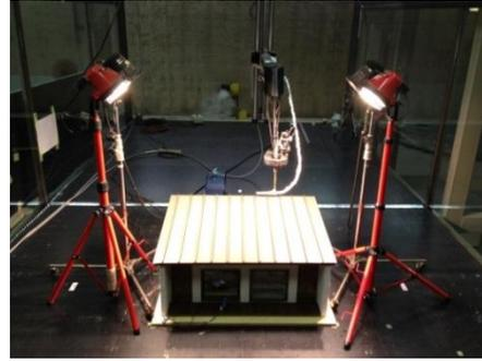
Fig. 2 Configuration of halogen lamps
