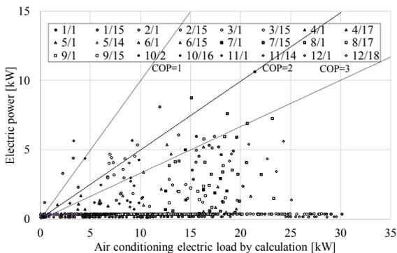
Fig.11 Comparison between air conditioning load calculated value and air conditioning electric power.
