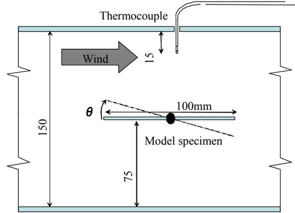
Fig. 5 Location of model specimen for evaluation of the effect of angle of attack.
