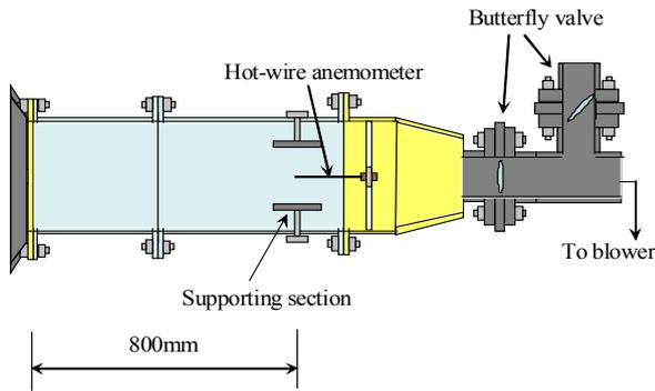
Fig. 1 Technical sketch of the experimental apparatus
