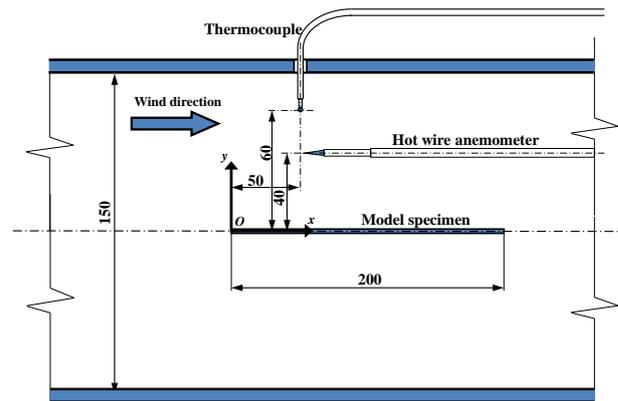
Fig.3 Location of the model specimen and measuring devices.
